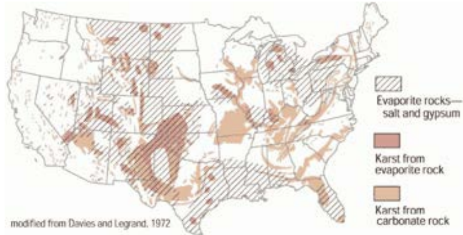
FIGURE G.11: UNITED STATES GEOLOGICAL SURVEY OF KARST MODIFIED FROM DAVIES AND LEGRAND, 1972
